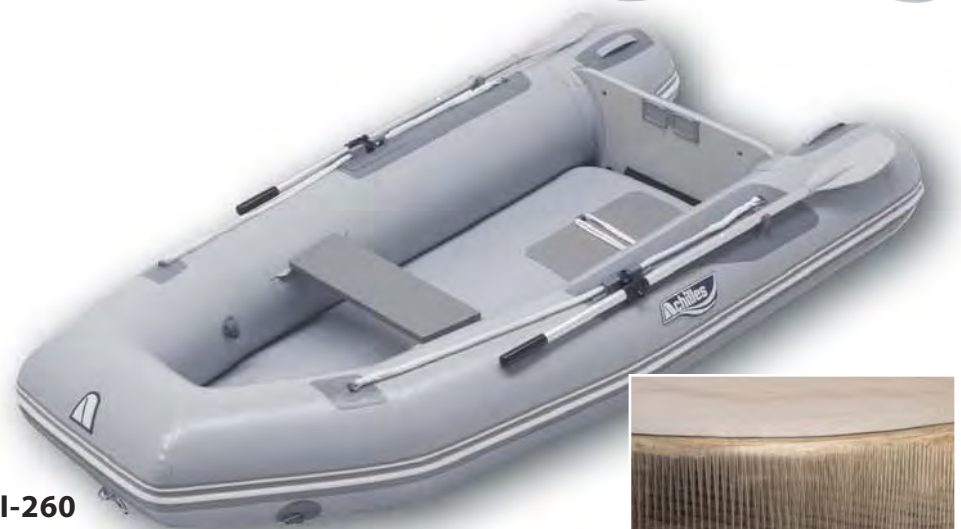
Achilles high-pressure, drop-stitch AirFirm™ floors provide superior rigidity.
